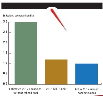
Emissions monitoring data show mercury emissions drop dramatically when CyClean refined coal is used to generate power from Associated's four cyclone units.
