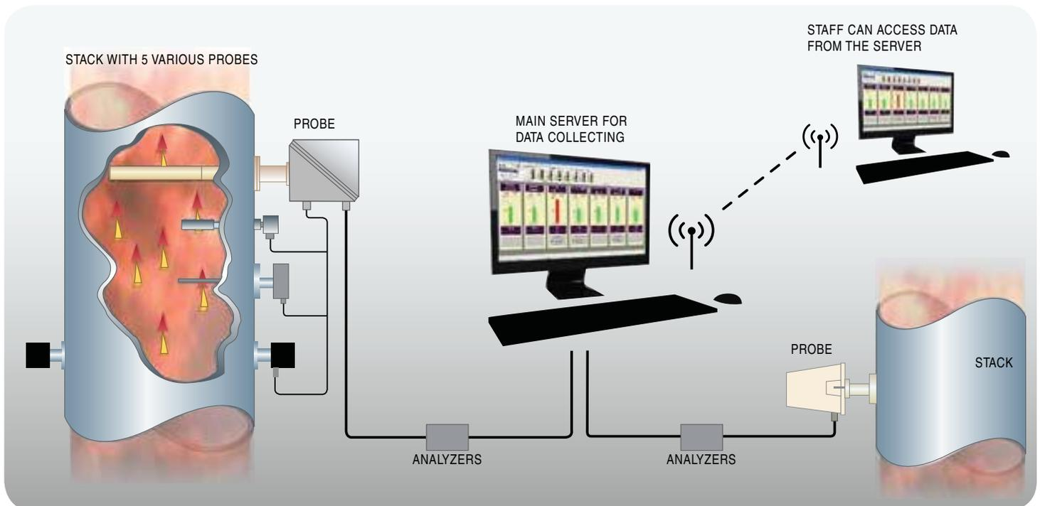
*Sensors on continuous emissions monitoring system probes in each power plant stack continuously record percentages of gas levels emitted. Emissions data from the analyzers are transmitted for calculation into tonnage for an accurate daily, weekly and monthly compliance report sent to state and federal agencies to ensure compliance with Associated's permitted air emissions limits.*
